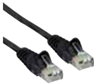
Network Cable CAT 5e UTP, AWG26 Copper, 50µ Gold Plated
