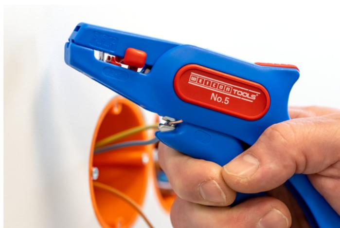
The WEICON Wire Stripper No. 5 is suitable for stripping all stranded and solid conductors from 0.2 – 6.0 mm<sup>2</sup>. The wire stripper also has a visual length scale from 5 - 12mm. The length stop can be removed, if required. A well-accessible side cutter is integrated in the tool, which is suitable for cable diameters up to 2 mm. The blades are replaceable. The low weight of the No. 5 ensures fatigue-free working.
