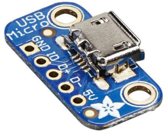
Simple but effective – this breakout board has a USB Micro-B connector, with all 5 pins broken out. Great for pairing with a microcontroller with USB support, or adding USB 5V power to a project.
