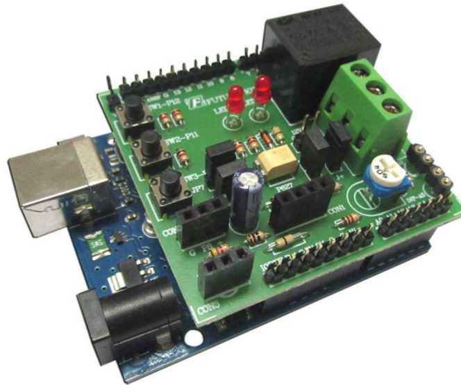
Figure 9. Connecting FK1413 board with Arduino UNO R3 board
