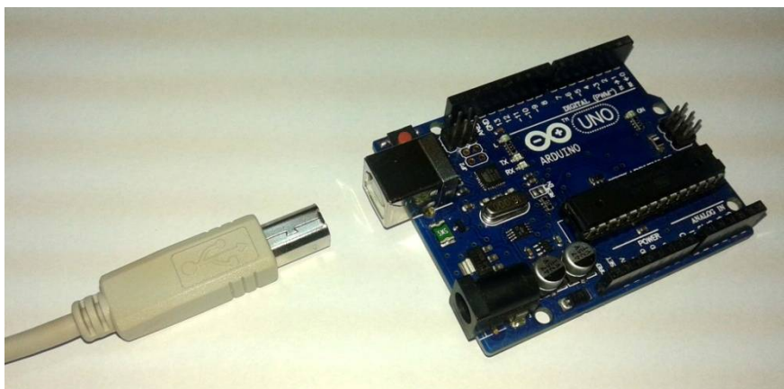
Figure 4. Connecting USB cable with USB port of Arduino Board
