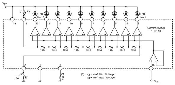
The above simplified TA7612AP Block Diagram is to give the general idea of the circuit's operation.
