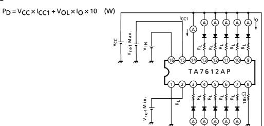
(Note)  $V_{OL}$  is :  $V_{OL} = V_{CC} - V_F$  (LED)  $- R_L \times I_O$  (When each output is "ON".)
